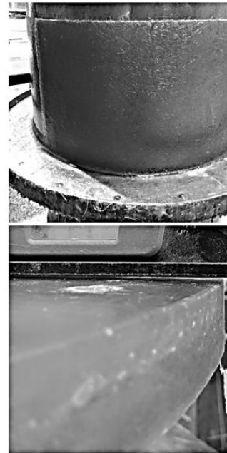
Figure 10: Derakane™ Signia™ 411 with CuNap manway on mold (top) and measure of flange drawback or curl after cure (bottom).
