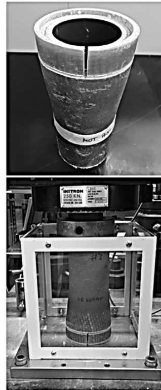
Figure 7. Machined M5 test specimen after machining (top) and M5 test specimen mounted in the Instron compression fixture (bottom).
