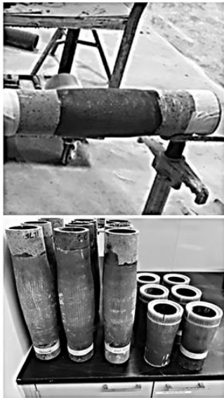
Figure 6. Preparation of M5 test specimens in a customer's shop (top) and pre-cut and machined M5 test specimens (bottom).
