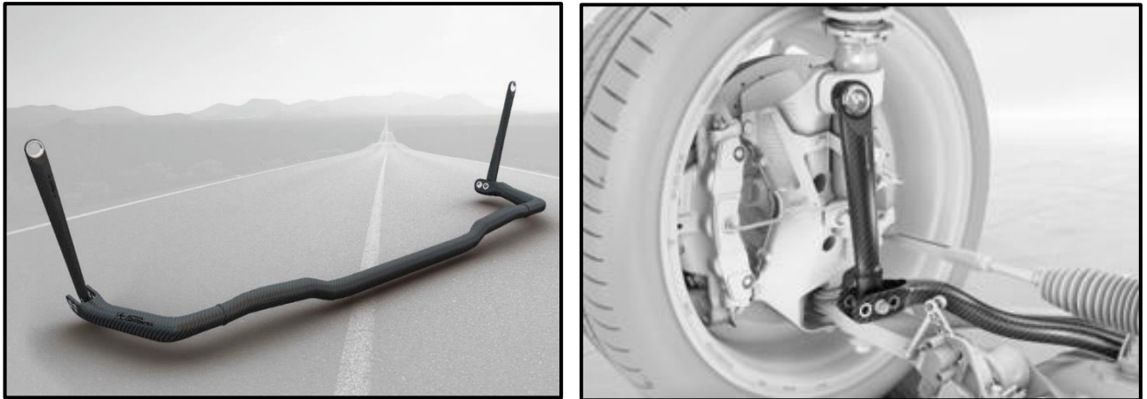
Fig. 5 The composite stabilizers on the front and rear axles
