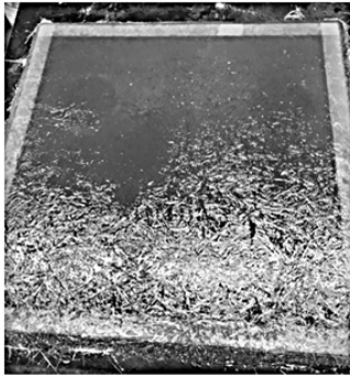
Figure 3. Picture of a completed secondary bonding test laminate with border tape separating the edge of the first and secondary layers.
