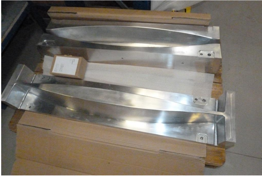
Fig. 7 Stamping tool for omega beam
