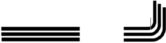
Fig. 4 Interlaminar sliding caused by laminate folding
