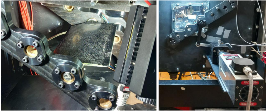
Fig. 4 Blade mounted in testing rig and test rig drive mechanism.
