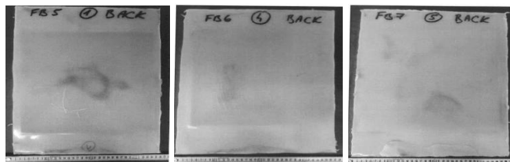
Fig. 5 Rear side of panels after tests
